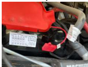
Solar Controller Fuse (colors vary red or black by year or model)
